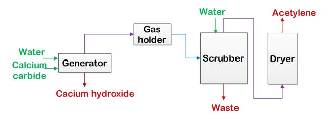
Figure: Manufacture of Acetylene by using Calcium carbide
